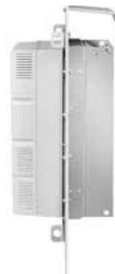
Flange mounting for panel installation ensures less thermal load inside panel by keeping most of the losses outside the panel.
